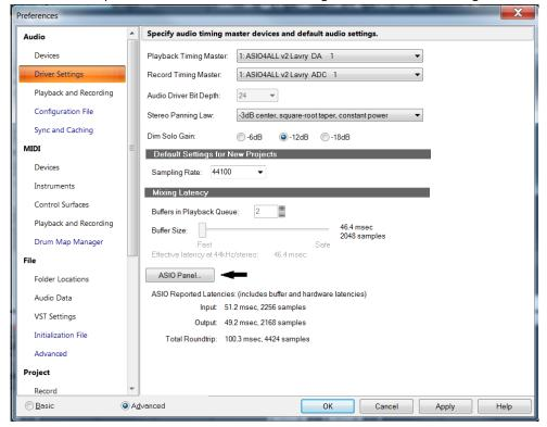
It may be necessary to close and re-open Sonar for the changes to appear in the Preferences Audio Devices or Audio Driver Settings dialogs after the Input and Output devices are changed in the ASIO Panel (ASIO4ALL Control panel).
