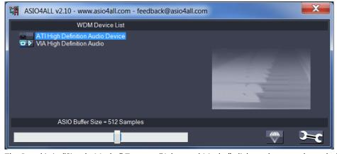
The Panel is in "Simple Mode." To open "Advanced Mode;" click on the wrench symbol in the lower right corner and the panel will change to show important settings.
